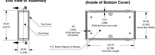
Front/Rear Panel (Dashed Line Indicates Viewing Area) [3.224] (Viewing Area) 26.50 29.00 [1.043] [1.142] (Viewing Area) [3.406] 1.65
